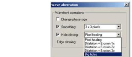
**Data map operations** such as smoothing, filtering or subtracting reference data adapt the shown results to your measurement setup.
